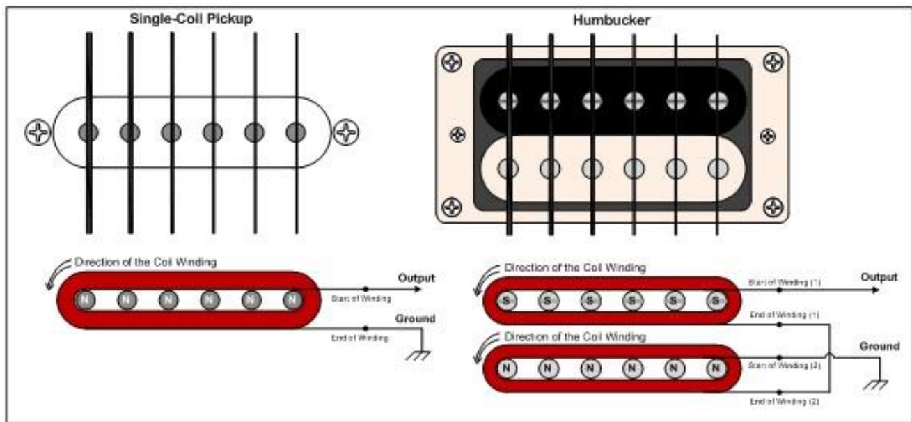
Slika 6 - Usporedba "Humbucker" i "Single coil" magneta
