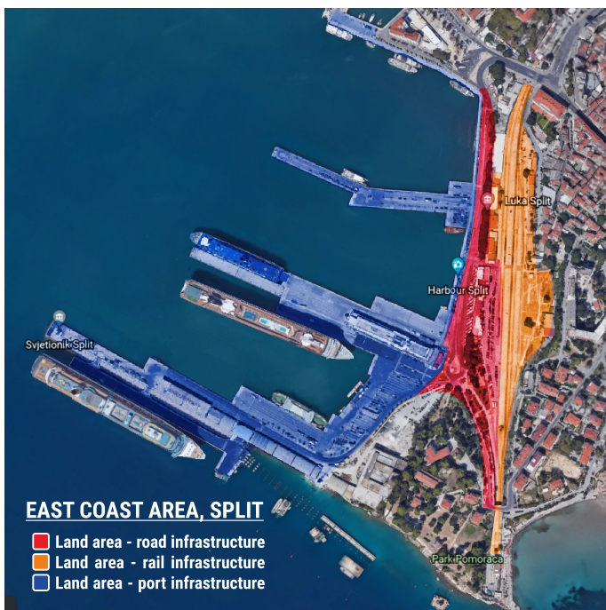
Figure 4.3: The land transport infrastructure area of East Coast Split, Google Maps (author's work)
